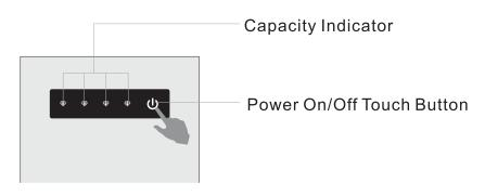
**Power On:** Press & hold the power on/off touch button for few seconds until the capacity indicators flash 3 times. The power on/off touch button light will keep flashing during the discharging. The Volt 9000 Duo will automatically power off when it idle for 1 minute.
