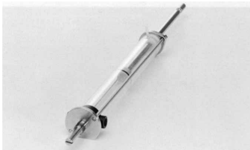
Fig 16. The cylinder package. Note that the tubing connectors are parallel to the flat surface on the end piece on the support rod assembly and that the rinsing tubing connector point upwards.
