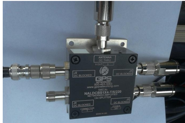
Figure 9 Splitter used to connect antennas
