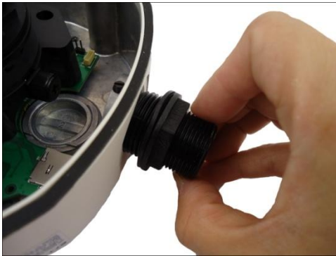
Attach to Side Conduit Hole
