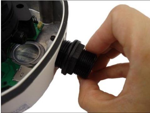
Attach to Camera Side Hole
