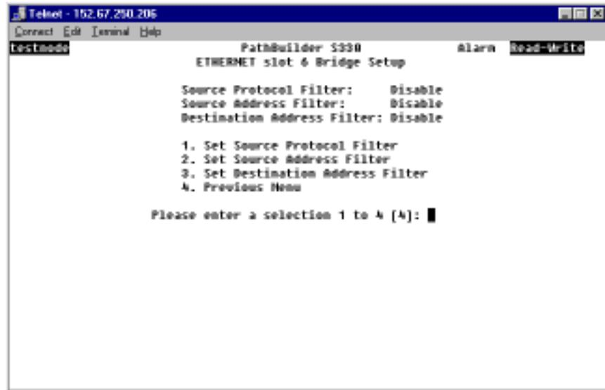
The current statuses of the source protocol filters are listed at the top of the menu. Yes indicates that packets with that protocol will be rejected. No indicates that packets with that protocol will be transmitted across the bridge.
