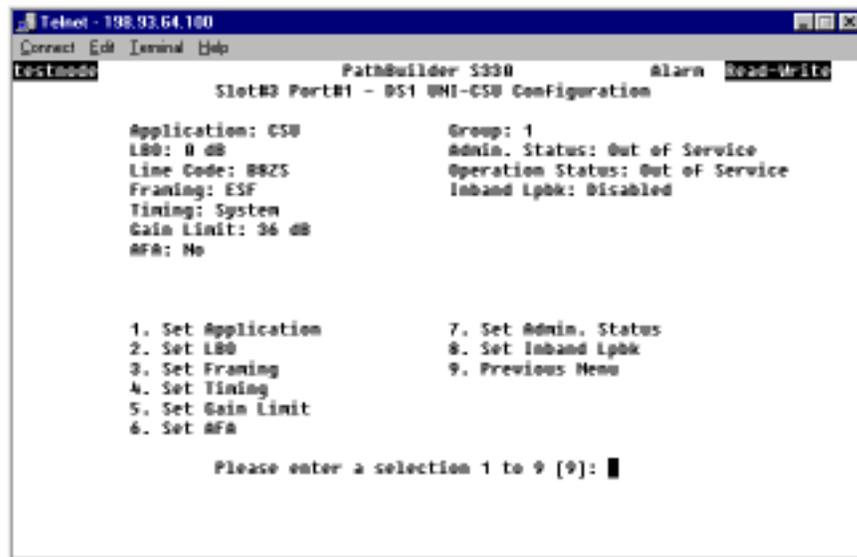
The Port Configuration menu lists the current parameters for the selected T1/E1 port and provides options for changing the settings.
