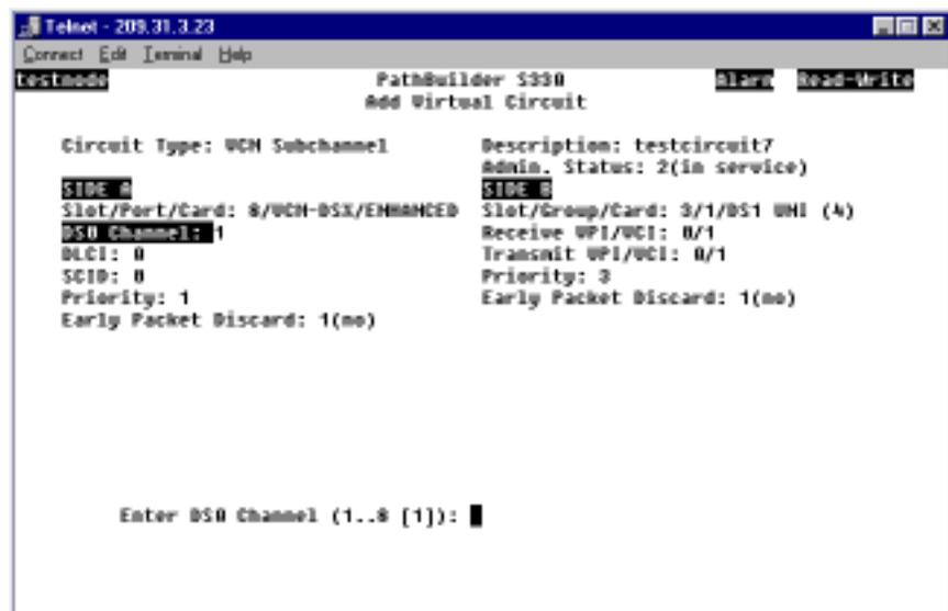
The VCM Subchannel Add Virtual Circuit screen lists the parameters for the selected VCM VCC circuit and prompts you to configure the subchannel parameters.
