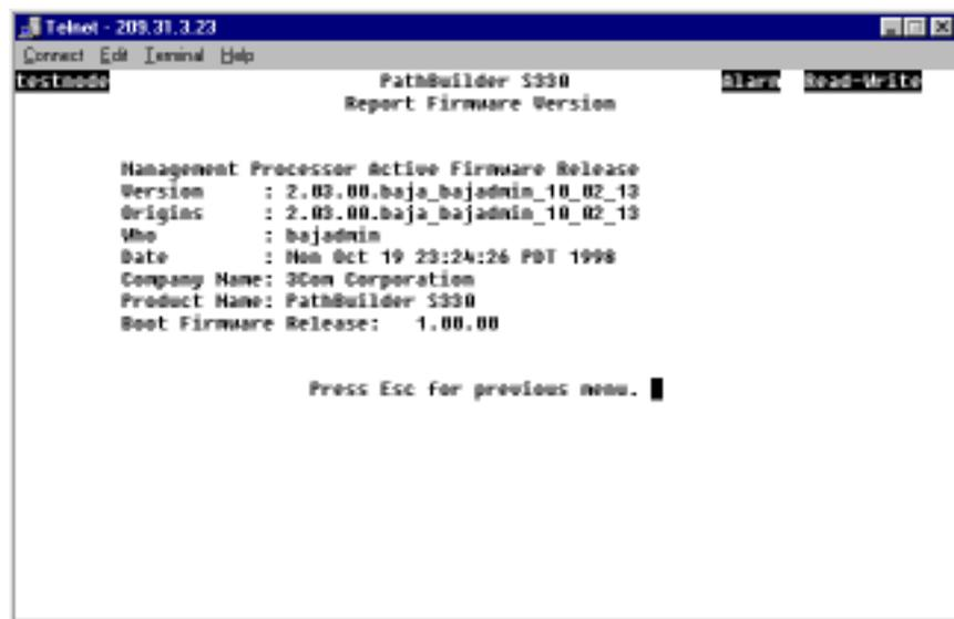
The Report Firmware Version screen displays the following information about the management processor active firmware (the upgradeable firmware currently being used by the MCP):
