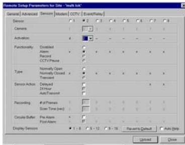
In this screen we can set the response of the system to each sensor. Functions that are not available in the unit you are using will be grayed out.
