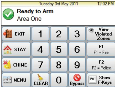
The top strip of the main screen displays the current time and date as programmed in the M1 Controller.
