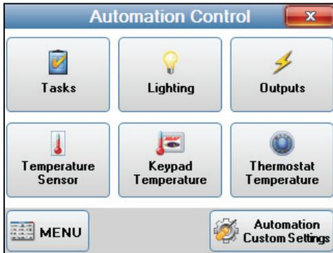
The Automation Control screen is displayed when the “**Automation button**” is selected in the Main Menu.
