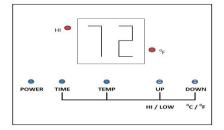
Press the <sup>o</sup>C/<sup>o</sup>F/Down to switch from Fahrenheit to Celsius.
