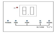
Press TIME to switch to time status, then press HI/LOW/UP button once within 5 seconds to scroll up
