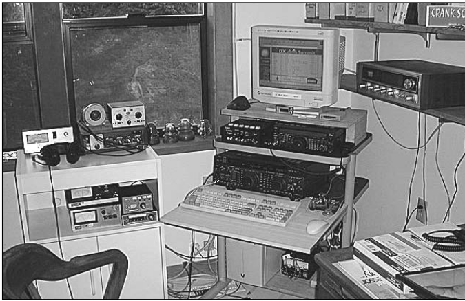
Fig 29.2 — Ward, N0AX, has had great success with this simple low power/QRP station tucked away in the corner of a room. All equipment fits on a computer cart and small rolling cabinet that make it easy to do station maintenance, as well as comfortable to use.
