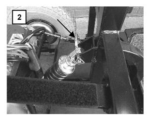
Secondly remove the locking pin located in the top of the rear shock absorber. Following this it is then necessary to disconnect the two loom connectors located in between the two battery trays so that the chassis can be separated. A picture of the loom connectors can be seen on the following page:
