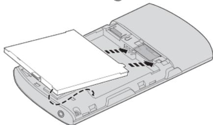
Insert the tabs on the bottom of the battery cover into the slots in the phone. Carefully press the top of the cover until the clips on the side of the cover click in place.
