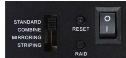
4. Once the enclosure has turned on, release the set "RAID button"..
