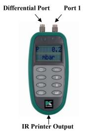
Always use the top right hand port (Port 1) for taking single channel measurements (pressure or vacuum). Only use the left hand port for differential measurements.
