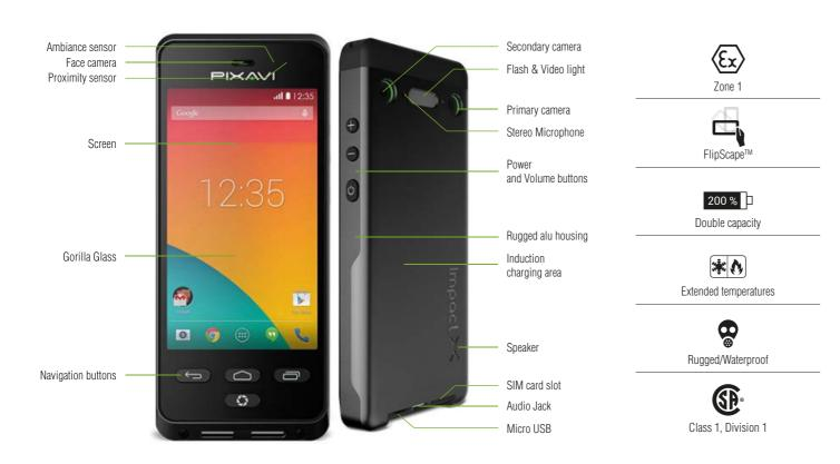
The BARTEC PIXAVI Impact X is the toughest smartphone you will ever meet. This intrinsically safe smartphone has all the functionality you will expect from a regular smartphone. The CSA Class 1, Division 1, IECEx and ATEX Zone 1 certification has not compromised the quality and usability. The device is explosion proof and rated for use in hazardous areas. The Impact X is the next generation wireless video communication technology from BARTEC PIXAVI.
