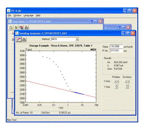
Note that the slope of the line and the value of pressure at 1 hour are shown and the permeability and skin have also been automatically calculated based on the position of the line. If you want to manually adjust the line, the slope and intercept can be entered. You can also change which points are active and fit another line to the data.
