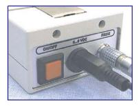
Fig. 5.4. AC/DC adaptor connection
