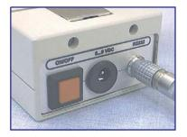
Fig. 5.3. RS-232 interface cable connection
