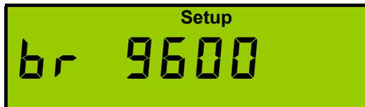
This sets the Baud Rate of the serial communications if the Modbus option is fitted at the factory.
