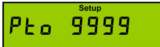
The pulse test facility allows the pulse output hardware and external system connections to be commissioned without a measured load. The LCD shows **Pto** (off) and **Ptr** (run) and the number of test pulses output. The test pulse rate is set automatically dependant on the programmed pulse length (maximum 0.5Hz).
