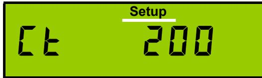
This should be set to match the nominal primary current rating, in Amps, of the external current transformers (CTs) fitted to the meter. The CT secondaries must match the nominal input rating of the meter (5A on standard meters).
