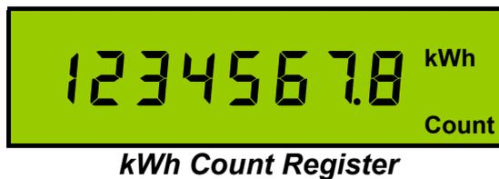
Scaling of the energy registers is set by the nominal input currents and voltages and remains constant during normal operation of the meter.
