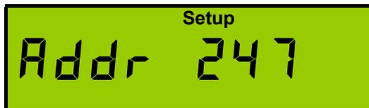
This sets the meters unique communications network ID (Modbus address) if the Modbus option is fitted at the factory.
