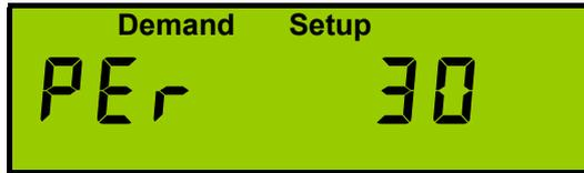
This sets the time, in minutes, over which kW Demand measurements are averaged. This is sometimes referred to as the sliding window or rolling average period.
