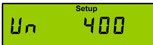
If no external Potential Transformer (PT) is fitted this is must be set to match the nominal line-line voltage (Un) of the meter as detailed on its rating label.
