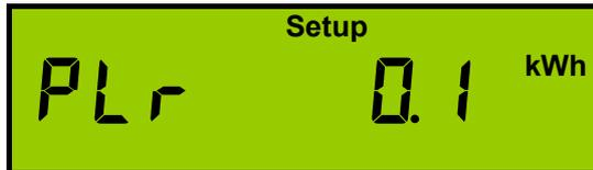
This sets the amount of energy measured between each pulse output. The scaling is dependant on the display scaling and therefore on the CT and PT programming.
