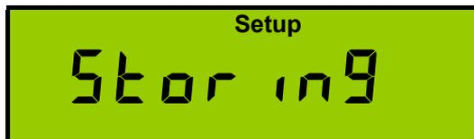
The programmed values are saved to non-volatile memory which is secure in the event of a loss of auxiliary power to the meter.
