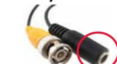
**Female Power Connector** - The female power connector (barrel) end of the Extension cable connects to the Power Adaptor.
