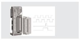
The CTRIO module has its own microprocessor and operates asynchronously with respect to the CPU. This means that on-board outputs respond in approximately 300µs to 2ms.
