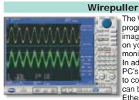
The Wirepuller software program displays a screen image of the DL's front panel on your PC so that you can monitor waveform signals. In addition, you can use the PC's mouse and keyboard to control the DL. The DL can be controlled via an Ethernet, USB, or GP-IB.
