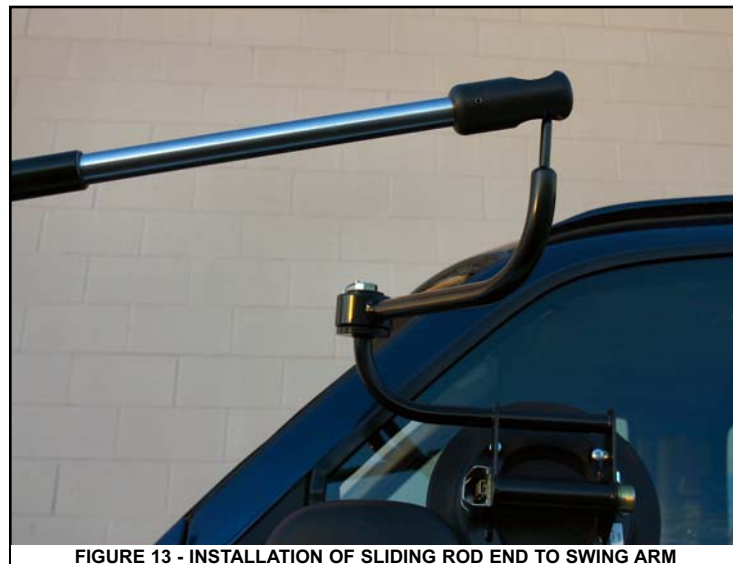
FIGURE 13 - INSTALLATION OF SLIDING ROD END TO SWING ARM
