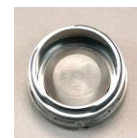
Properly installed Pirelli exhaust valve diaphragm (outer cover of exhaust valve not shown)
