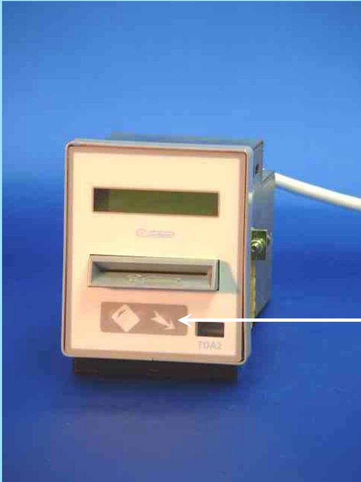
**Push Any of the Three Membrane Buttons in the Gray Rectangle to Request Card Ejection**
