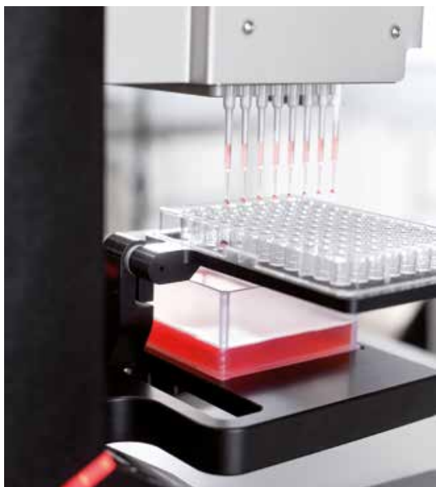
Single rows (e.g. to produce serial dilutions) can be pipetted easily due to 8 channel magazine
