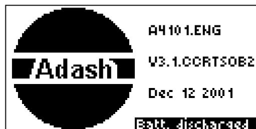
Fig. Signalling of discharged cells
