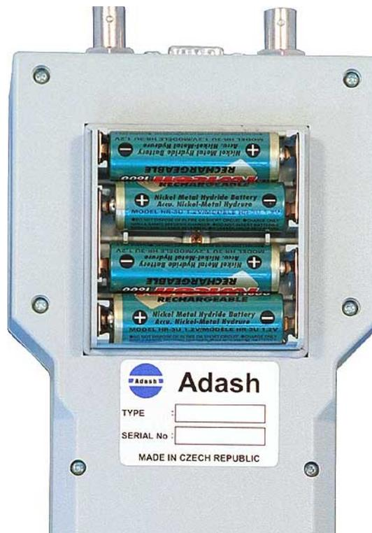
Fig. Correct polarity of the supply cells
