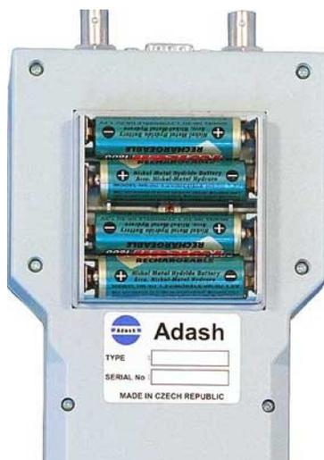
Fig. Correct polarity of the cells
