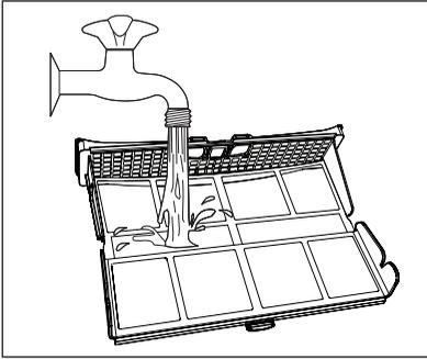
5. If necessary clean the filter with warm water using a brush.
