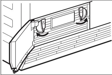
3. Turn the 2 blockages to unlock the condenser lid.
