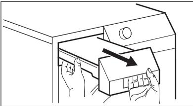
1. Pull the condensed water container and keep it in horizontal position.
