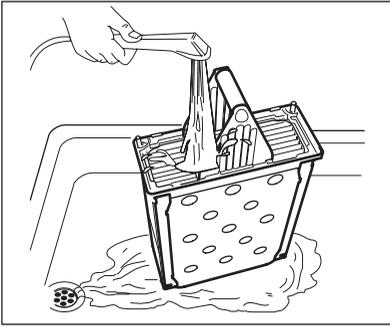
6. Clean the condenser in vertical position over a basin or paddling. Rinse through with a hand shower.
