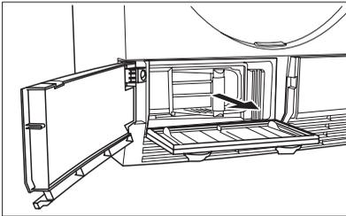
5. Catch the handle and pull the condenser out from the bottom compartment. Move condenser horizontally to do not spill remaining water.
