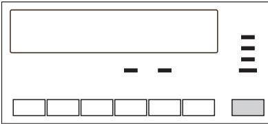
To activate the programme push the Start/Pause button. The LED above the push button changes the colour to red.
