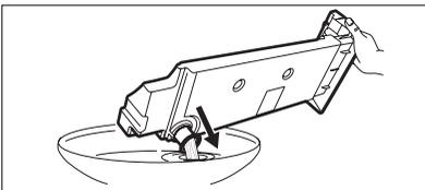
2. Move the plastic connection out and drain the condensed water container into a sink or equivalent receptacle.
