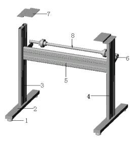
Step 5: Lay down the four pillars of main machine, place the machine on the connection board, then insert the pillars into the connection board to connect to the main machine.
