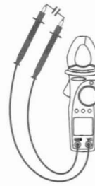
Fig. 9: use of clamp for continuity measure
