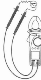
Fig. 5: Use of clamp for AC/DC uA current measures
