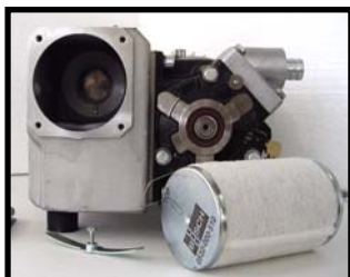
Remove tensioner and filter from the housing
