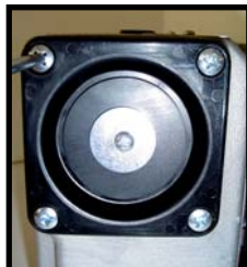
Screw the cover from the filter housing
