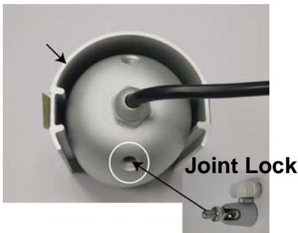
3. Screw the camera with the Joint Lock connected to the bracket. Adjust the camera angle and the Sun Shield position. After that, secure the Joint Lock to fix. Then, pass the Power and Video Cable through the hole drilled in Step 1 to hide it.
