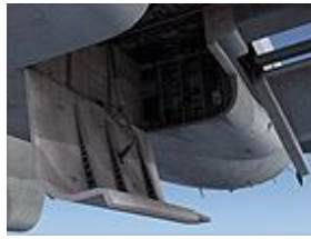
Service access doors
