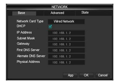
[DHCP]: Enable the DVR to obtain an IP address automatically. If this is enabled, the DVR will reboot and search for a DHCP server, and then assign a dynamic IP address. The dynamic IP address will be displayed in the menu. Enter a static IP address if there is no DHCP service available. If you are using the advanced feature PPPoE, then the IP/mask/gateway and DHCP are unable to be changed.
