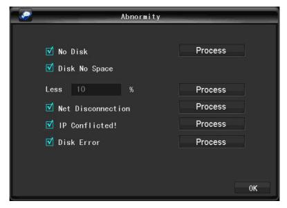
[No Disk] Alarm when the hard disk is not present or can not be detected. [Process Mode] includes: [Alarm Output], [Display On Screen] and [Send Email].
