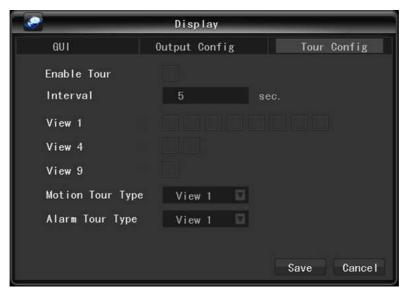
Setting tour mode and interval between rotation, the time is within 5-120s, the mode include single screen, four-, eight-, nine-, sixteen-screen.
