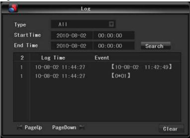
Log type: System operation; configuration; data management; alarm event; recording; user management; log delete; document operation. Select the type and time to filter the log list. Backup logs by clicking "backup" or clicking "delete" to delete all logs.
