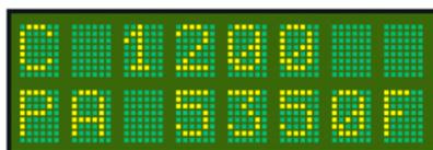
**5350 FEET.** Units in feet are indicated by the **F** character at the right hand end of the lower display line. All altitude data will be displayed in feet.
