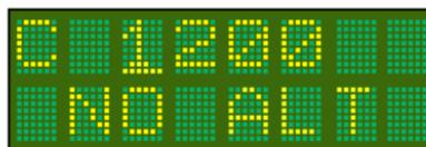
It is possible to input the **QNH / Baro** (barometric pressure) given by ATC, into the **T2000** to adjust the displayed pressure altitude. This feature will allow the user to adjust the displayed altitude to read the same as the aircraft's altimeter.
