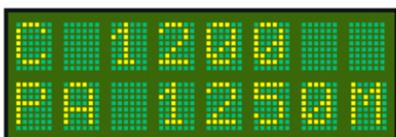
**1500 METRES.** Units in metres are indicated by the **M** character at the right hand end of the lower display line. All altitude data will be displayed in metres.
