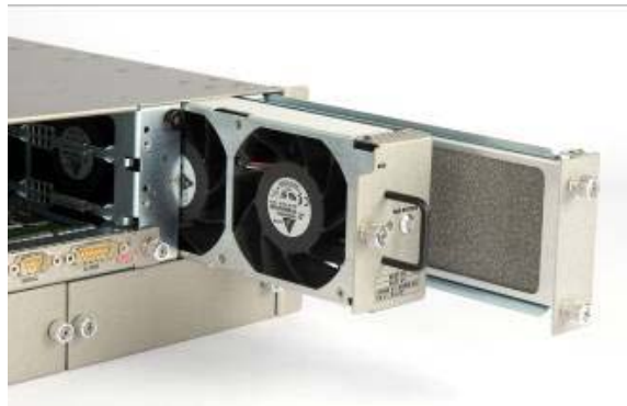
Figure 20 – Extracting a Fan Tray
