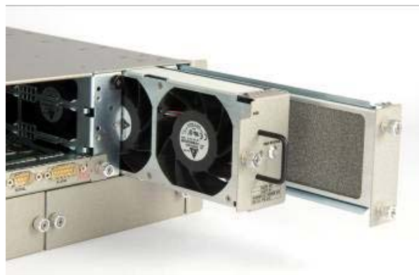
Figure 16 - Fan and Air filter trays
