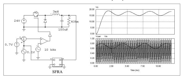
The simulated waveforms of the load voltage, modulation wave and the carrier wave are shown on the right.
