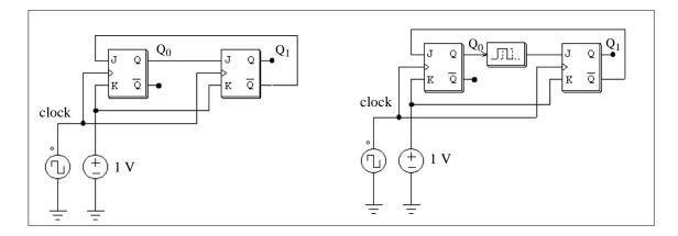
In the circuit on the left, the initial values of both Q0 and Q1 are assumed to be zero. At the clock rising edge, Q0 will change to 1. Without delay, the position of Q1, which should remain at 0, will toggle to 1 at the same time.
