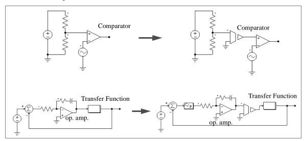
It should be noted that, in PSIM, the power circuit and the control circuit are solved separately. There is one time step delay between the power and the control circuit solutions.
