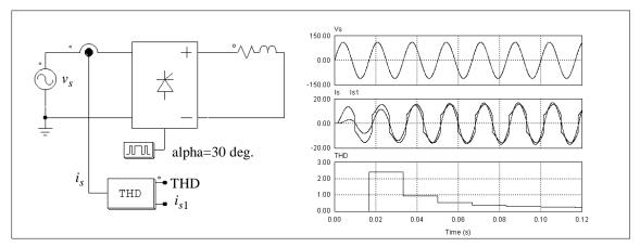
One of the THD block output is the input current fundamental component  $i_{s1}$ . By comparing the phase difference between the input voltage  $v_s$  and the current  $i_{s1}$ , one can calculate the input displacement power factor. This, together with the THD value, can be used to calculate the input power factor.
