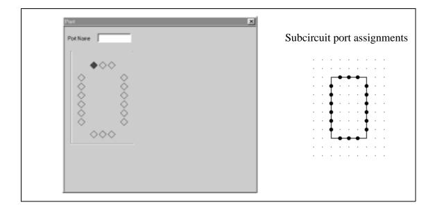
The diamonds on the four sides represent the connection nodes and the positions of the subcircuit. They correspond to the connection nodes of the subcircuit block on the right. There are no diamonds at the four corners since connections to the corners are not permitted.
