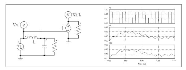
The voltage source is controlled by the branch current  $i_s$ . With a gain of 1, the waveform of the voltage  $v_{is}$  is identical to that of  $i_s$ .
