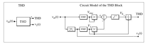
A second-order band-pass filter is used to extract the fundamental component. The center frequency and the passing band of the band-pass filter need to be specified.
