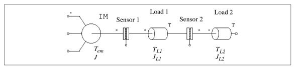
The system consists of one machine, 2 torque sensors, and 2 mechanical loads. The torques and moment of inertia for the machine and the loads are as labelled in the diagram. The reference direction of this mechanical system is from left to right. The equation for this system can be written as:
