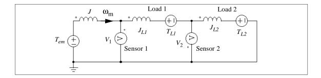
The current in the circuit represents the mechanical speed  $\omega_{\rm m}$ . The voltage probe  $V_1$ , which measures the node-to-ground voltage at the machine shaft output, represents the reading of the torque sensor No. 1. Similarly, the probe  $V_2$  represents the reading of the torque sensor No. 2. Note that the probe  $V_2$  is inverted (from the ground to the node) since Sensor 2 is against the reference direction of the mechanical system.
