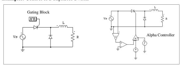
This circuit on the left uses a switching gating block (see Section 2.2.4). The switching gating pattern and the frequency are pre-defined, and will remain unchanged throughout the simulation. The circuit on the right uses an alpha controller (see Section 4.7.2). The delay angle alpha, in degree, is specified through the dc source in the circuit.
