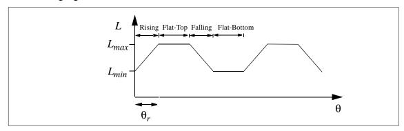
The rotor angle is defined such that, when the stator and the rotor teeth are completely out of alignment,  $\theta = 0$ . The value of the inductance can be in either rising stage, flat-top stage, falling stage, or flat-bottom stage.
