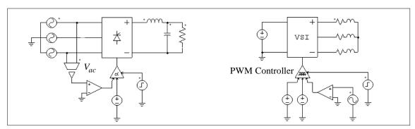
The thyristor circuit on the left uses an alpha controller. For a three-phase circuit, the zero-crossing of the voltage  $V_{ac}$  corresponds to the moment when the delay angle alpha is equal to zero. This signal is, therefore, used to provide synchronization to the controller.
