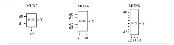
In the images, d0..d7 are the data inputs; and s0..s2 are the control signals. The truth tables of the multiplexers are:
