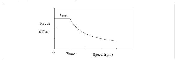
When the mechanical speed is less than the base speed  $n_{\text{base}}$ , the load torque is:
