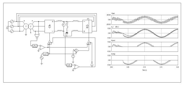
The simulated waveforms of the load voltage, load current (before and after the band-pass filter), and the currents through the positive and negative rectifier bridges are shown below:
