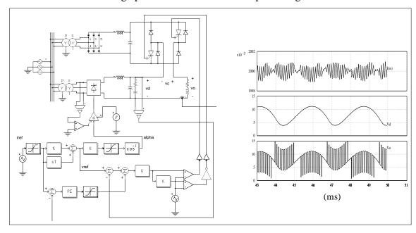
The simulated waveforms of the load current, rectifier voltage (after the low-pass filter), and the load voltage are shown.
