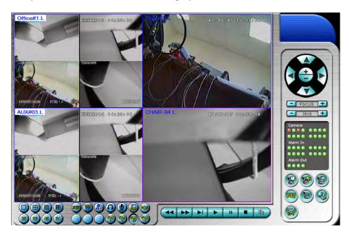
The video images can be displayed in several types of split-window screens, including 1/4/9/16-Window for single DVR and 25/36/49/64 for multiple DVRs. And the focus window is surrounded by a frame border. In addition to the video windows, there are different icons on the lower corner and the right corner of the screen for status display and control. (The ".L" following the camera title stands
