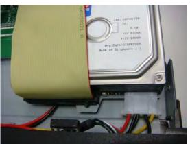
4. Use the tape to fix the flat cable connectors firmly, esp. for ISD-204.
