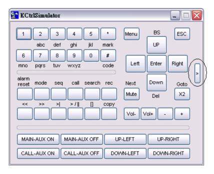
Please note that most of the buttons correspond to the keypads on the front panel. If you connect the PC through RS-232 and use an RS-232/RS-485 converter to connect to multiple DVRs, you would be able to control multiple DVRs via the simulation software. Please refer to Section 3.2 Optional Connections to connect/cascade the DVRs to the PC.
