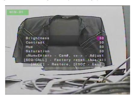
There are 4 items which can be adjusted, including Brightness, Contrast, Hue, and Saturation. The operations are as below:
