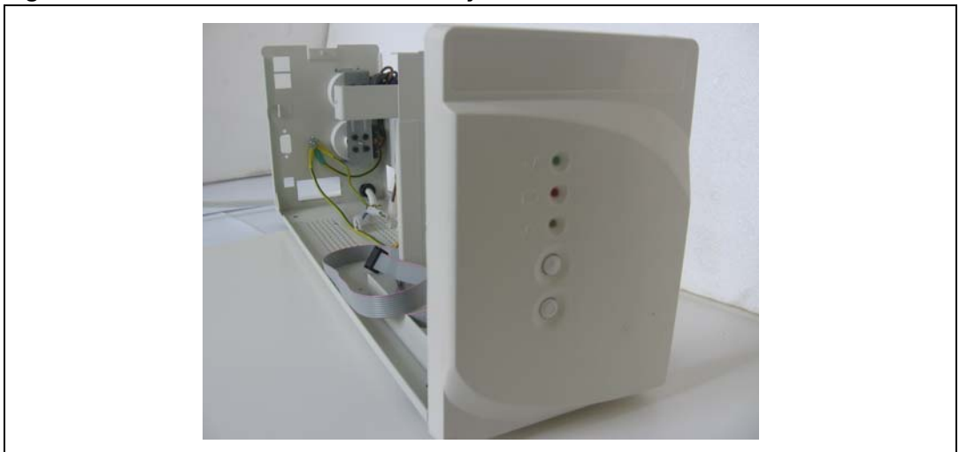
Figure 30. UPS with batteries and battery fuse
