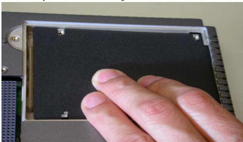
Figure E.19: Laying in the HDD insulator
