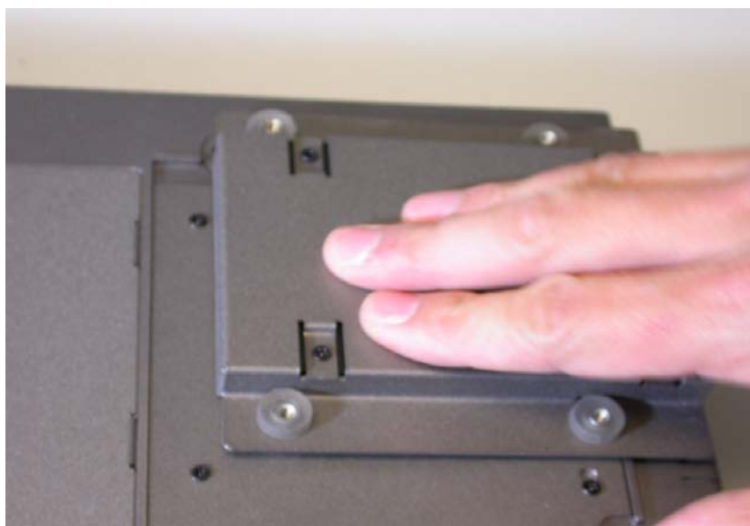
Figure E.12: Placing the HDD holder - 2
