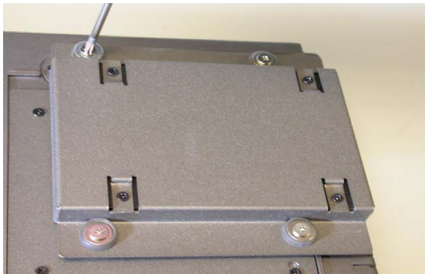
Figure E.13: Fastening the HDD holder
