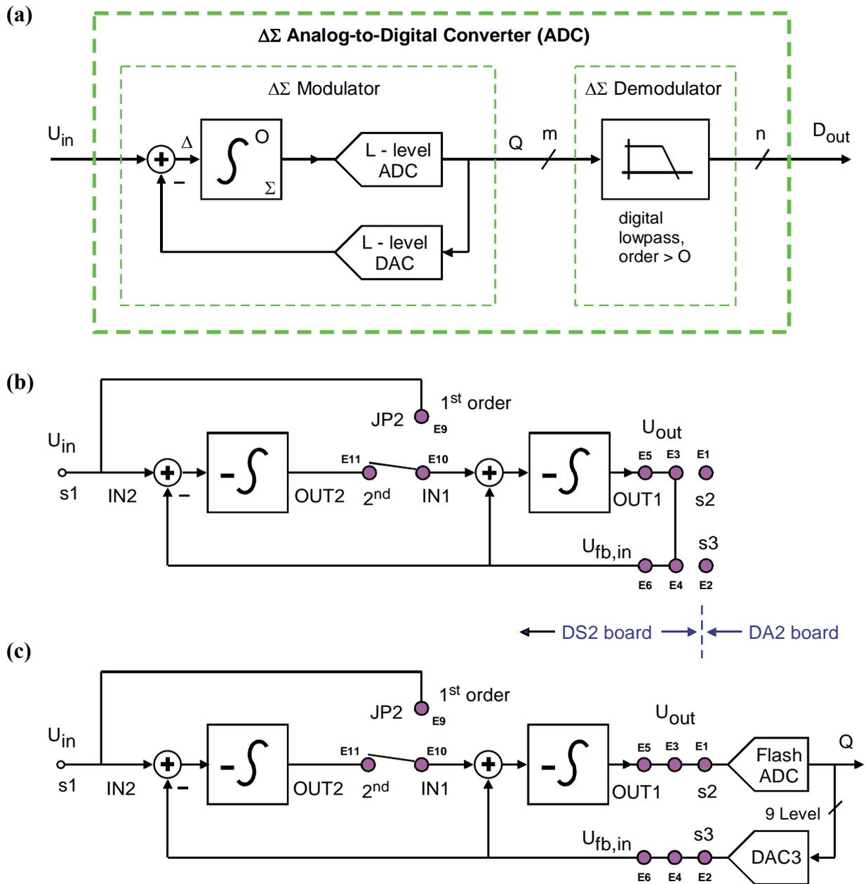
**Fig 6.3.4-1:** (a) Principle of using  $\Delta\Sigma$  Modulation for A/D Conversion. (b) Analog integrator loop of DS2 board. (c) Incorporation of ADC and DAC makes analog loop to  $\Delta\Sigma$  modulator.
