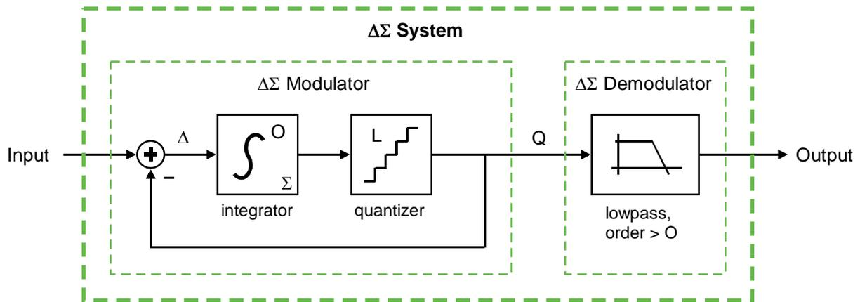
**Fig 6.3.2:** Principle of  $\Delta\Sigma$  Modulation: An  $O^{\text{th}}$  order integrator and a quantizer within a loop
