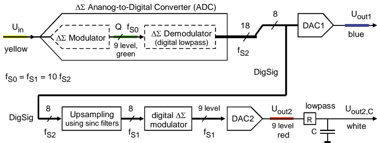
**Fig 6.1:** The complete system: A  $\Delta\Sigma$ -ADC feed two DACs: *DAC1* and *DAC2*.
