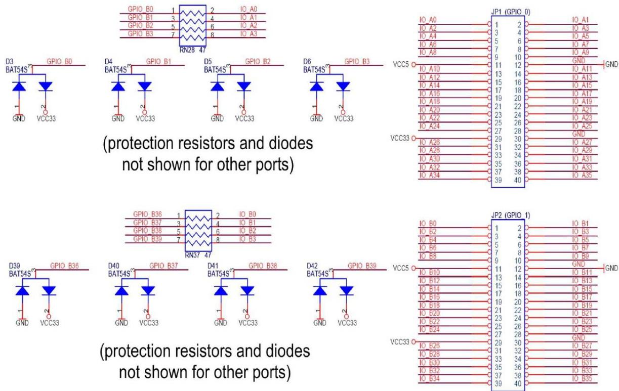
Figure 4.10. Schematic diagram of the expansion headers.
