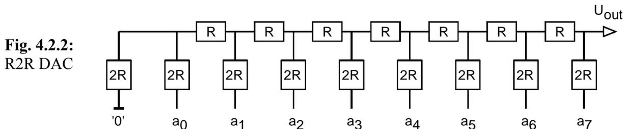
The R2R ladder DAC with output  $DAC1_{out}$  delivers an output voltage of
