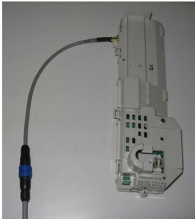
Fig. 41. Board with appliance cable connected
