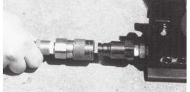
While holding RABBIT TOOL in place, activate tool by turning pump relief valve knob toward hose and pumping handle up and down.
