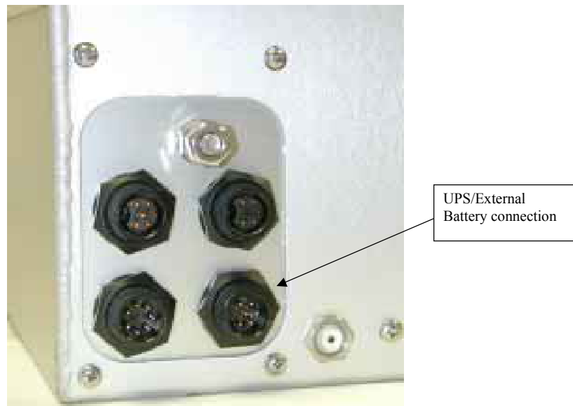
Figure 6 USP/External Battery connection.
