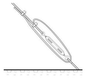
Step six. Adjust turnbuckles. A little loose tightwire is safe than a tight one.
