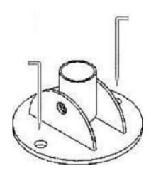
Note: If the ground is loose, please make concrete base for tower base and anchors (depth=500mm, length=400mm).
