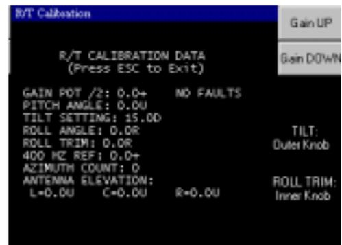
If the radar R/T was already calibrated prior to FSD installation, enter the roll trim value that was previously written down, using the inner knob. Press Enter to accept the new values.
