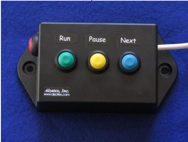
The remote inputs are ground closure type. The **Run**, **Pause** and **Stop** inputs are typically connected to operator buttons. The **Increment (Next)** button may be a button for the operator or may be connected directly to a machine trigger.
