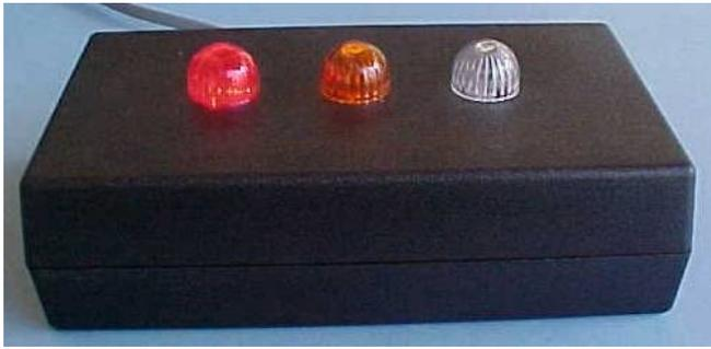
These warnings can be used to indicate whether the actual time is longer or shorter than the TAKT time and determine whether there is a problem with production or whether a particular operator is slower or faster or whether the TAKT time is too long or too short.
