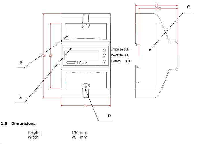
Depth65 mmMax diameter cable11.5 mm (7.5mm with adaptor 1 and 4.9mm with adaptor 2)Weight0.2 Kg (net)
