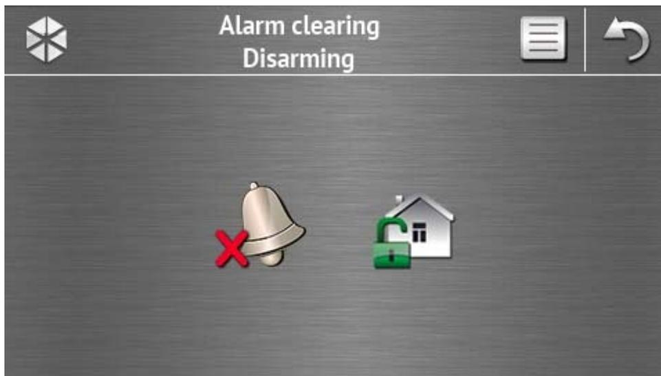
The “Alarm clearing / Disarming” screen will be displayed after you tap the
