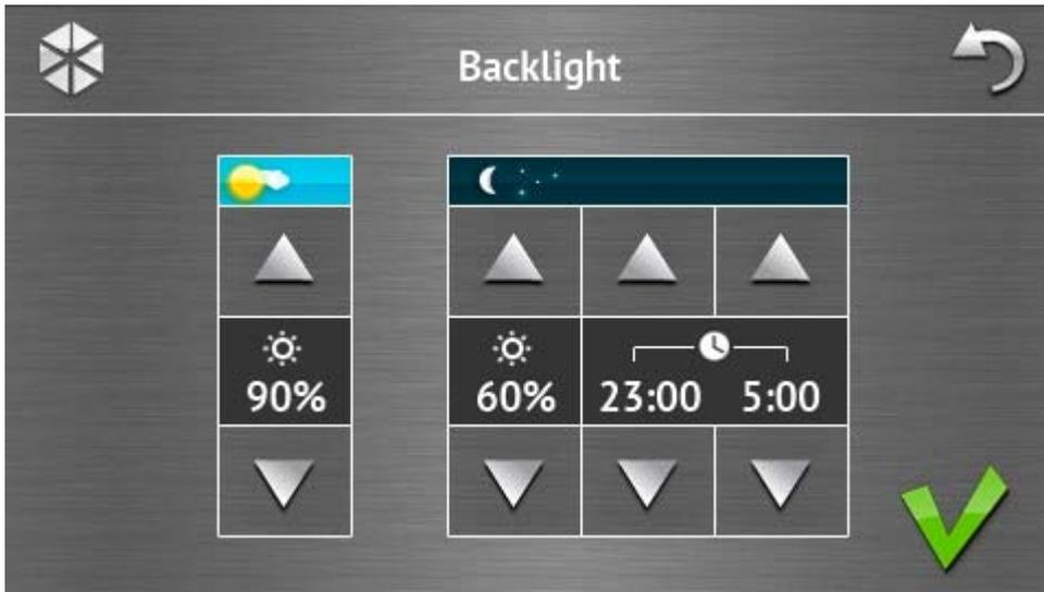
Intensity of the screen backlight can be controlled within the 10-100% range. In the night hours, which can be specified, the backlight intensity can be different.
