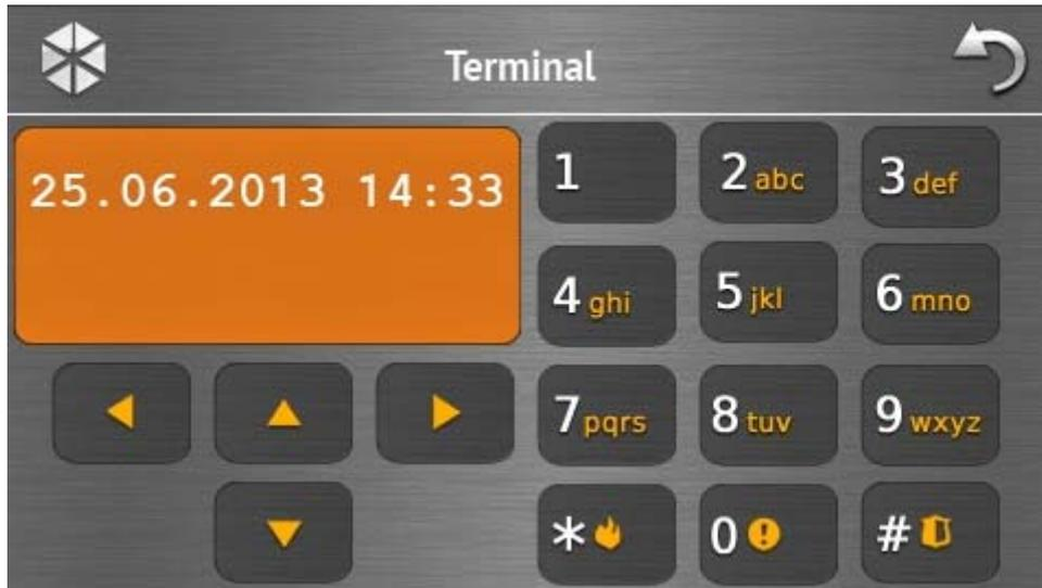
The terminal enables the alarm system to be operated and programmed in the same way as from the LCD keypad with text menu. The method of using such a keypad is described in the control panel programming / user manuals (electronic versions of the manuals are available on the [www.satel.eu](http://www.satel.eu) website).
