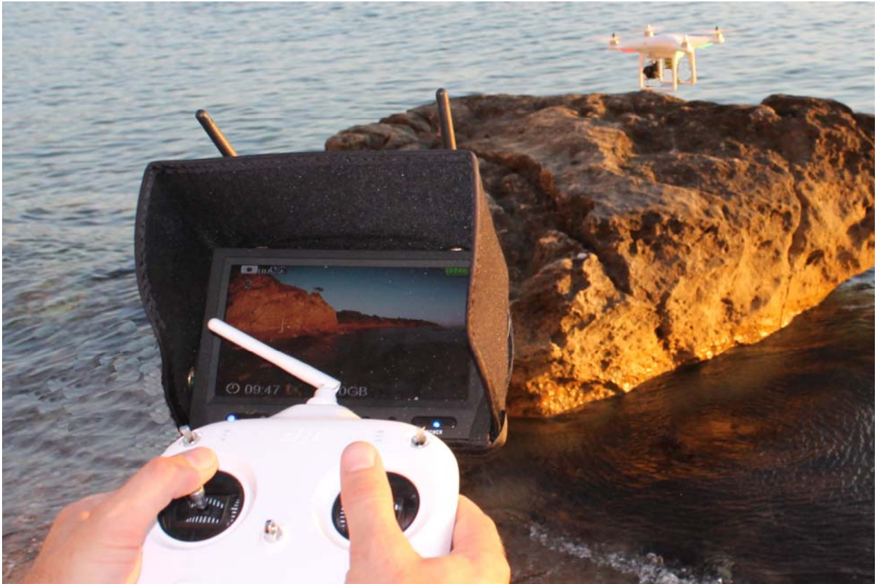
DJI Phantom + CamOne infinity + 5,8 GHz Transmitter Set and 7" (178mm) Diversity Screen
