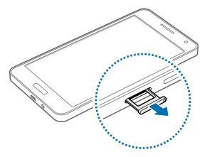
Place the SIM or USIM card in the SIM card tray with the gold-coloured contacts facing downwards.
