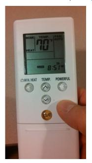
**Avoid "Auto" mode** - Set your heat pump mode to "Heat" in the winter and "Cool" in the summer, but avoid using the "Auto" mode. Auto mode could inadvertently turn on heating during a cool summer night or air conditioning on a sunny winter afternoon.
